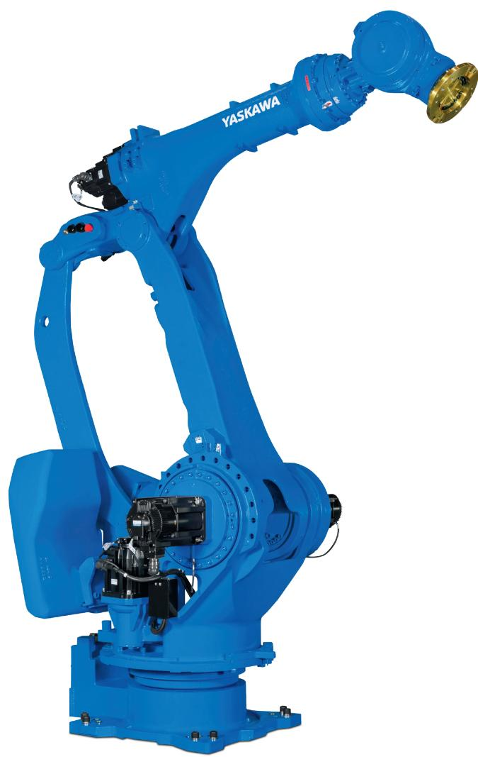
The MOTOMAN GP360 6-axis robot is a powerful and versatile industrial robot that is ideal for a wide range of applications. The product features a high payload of 360 kg and a large working range.
